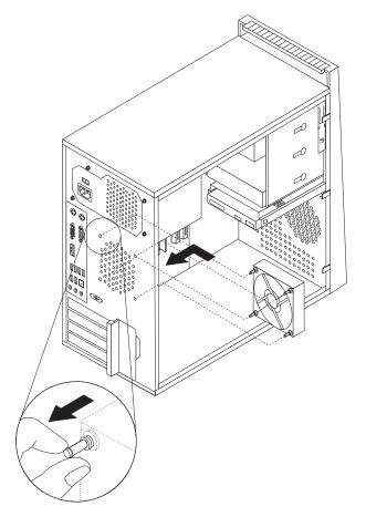
Figure 34. Installing the rear fan assembly
